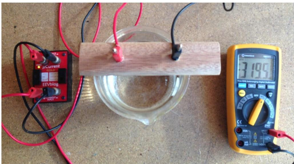
The bottom and top probes in the image above have a copper wire (3mm diameter) extending from the electrode (probe) connector through to the central column. A separation of the top and bottom probes by about 5-6 cm seems to provide less interference or more stability in the reading. Usually a stable reading is obtained after about 1 minute where it may fluctuate between negative and positive before settling down to a steady (negative charge) measurement state.
