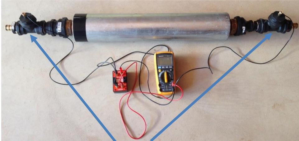
Two inline copper probes (electrodes or voltage detectors) units are required for this measurement, as illustrated in the image above.
