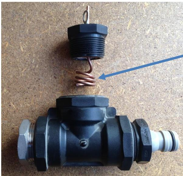
The electrode (3mm copper coil) should be long enough to fit just above the bottom of the unit and within the flow of the water. Banana or alligator connectors from the UCurrent device can be used to attach to the copper electrode.
